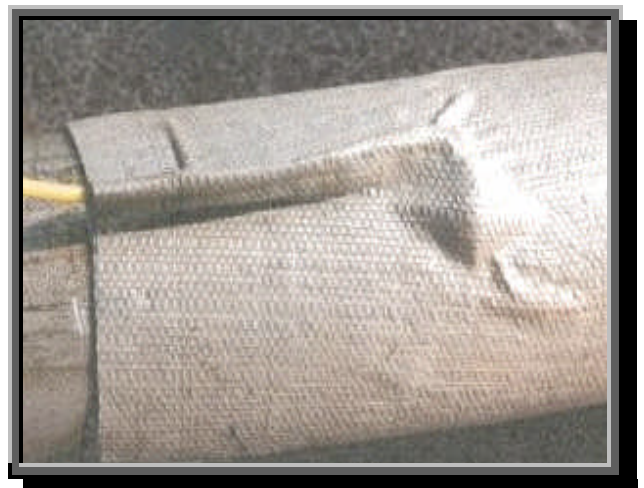
Figure 1-2. The above photo illustrates how one competitor's coating can emphasize an already weakened coating on a weld "load" point
