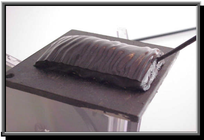
Figure 1-4. Thermite weld coated with the KEMA 250-12 Module Sealant system.
