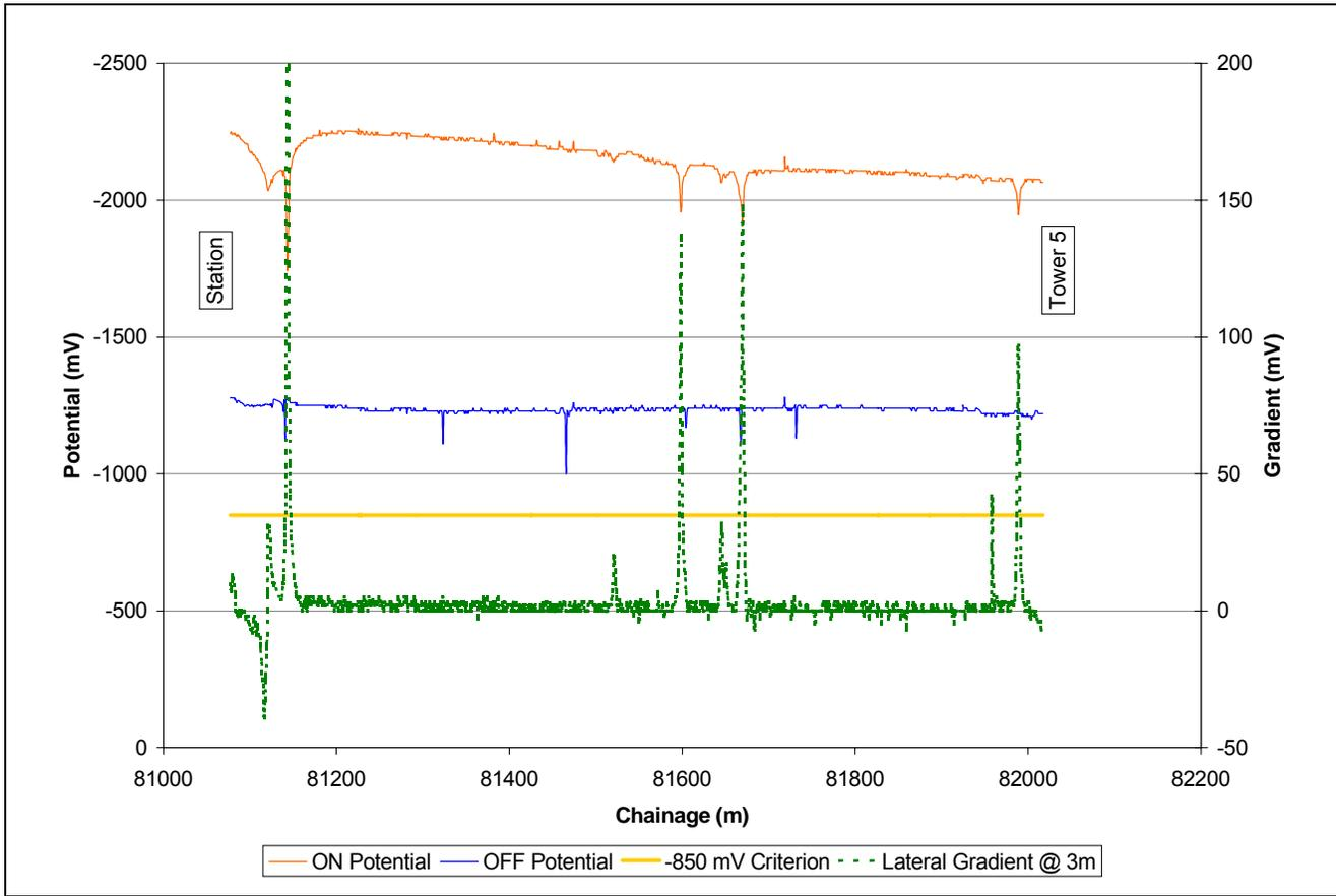
**Figure 4. 16" Pipeline. CIPS/DCVG Survey. (1.1 Km Sample)**
