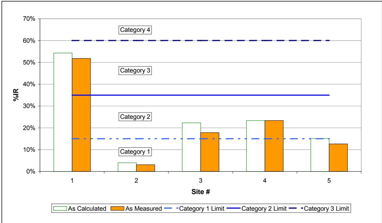
**Figure 7. Comparison between “As Measured” and “As Calculated” %IR**
