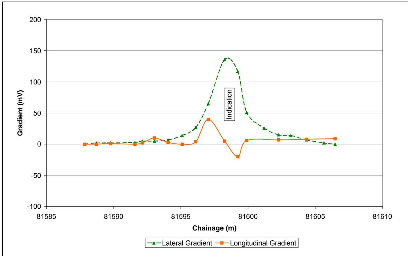
**Figure 8. 16" Pipeline. Chainage 81598m. Voltage Gradients at DCVG Indication**
