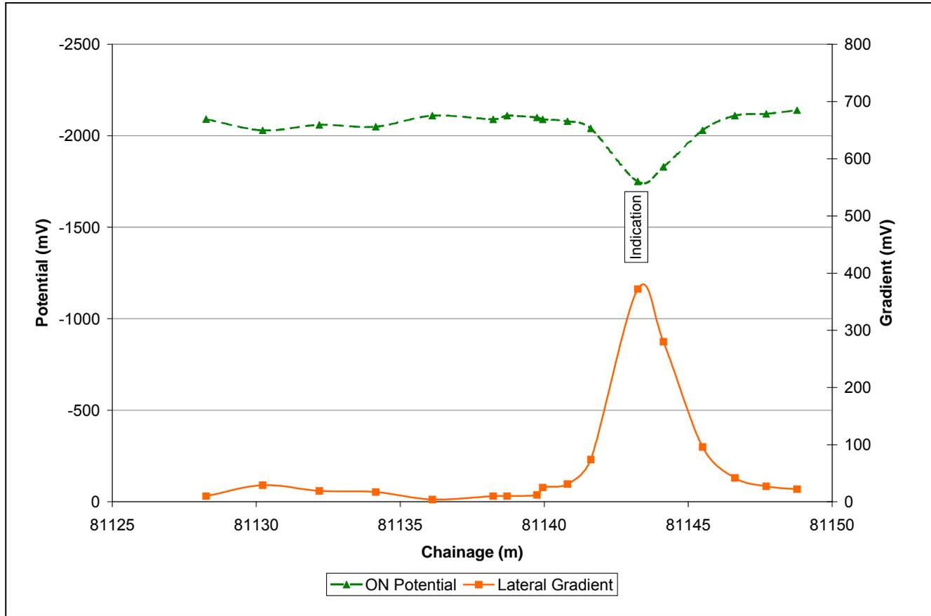
**Figure 3. 16" Pipeline. Identification of Indications Based on Potential and Gradient Profile**
