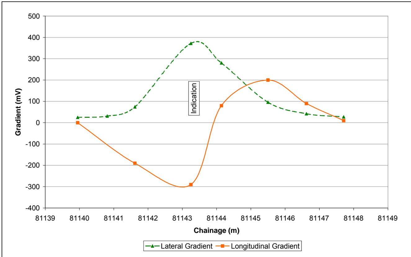
**Figure 2. 16" Pipeline. Chainage 81143.25m. Voltage Gradients at DCVG Indication**
