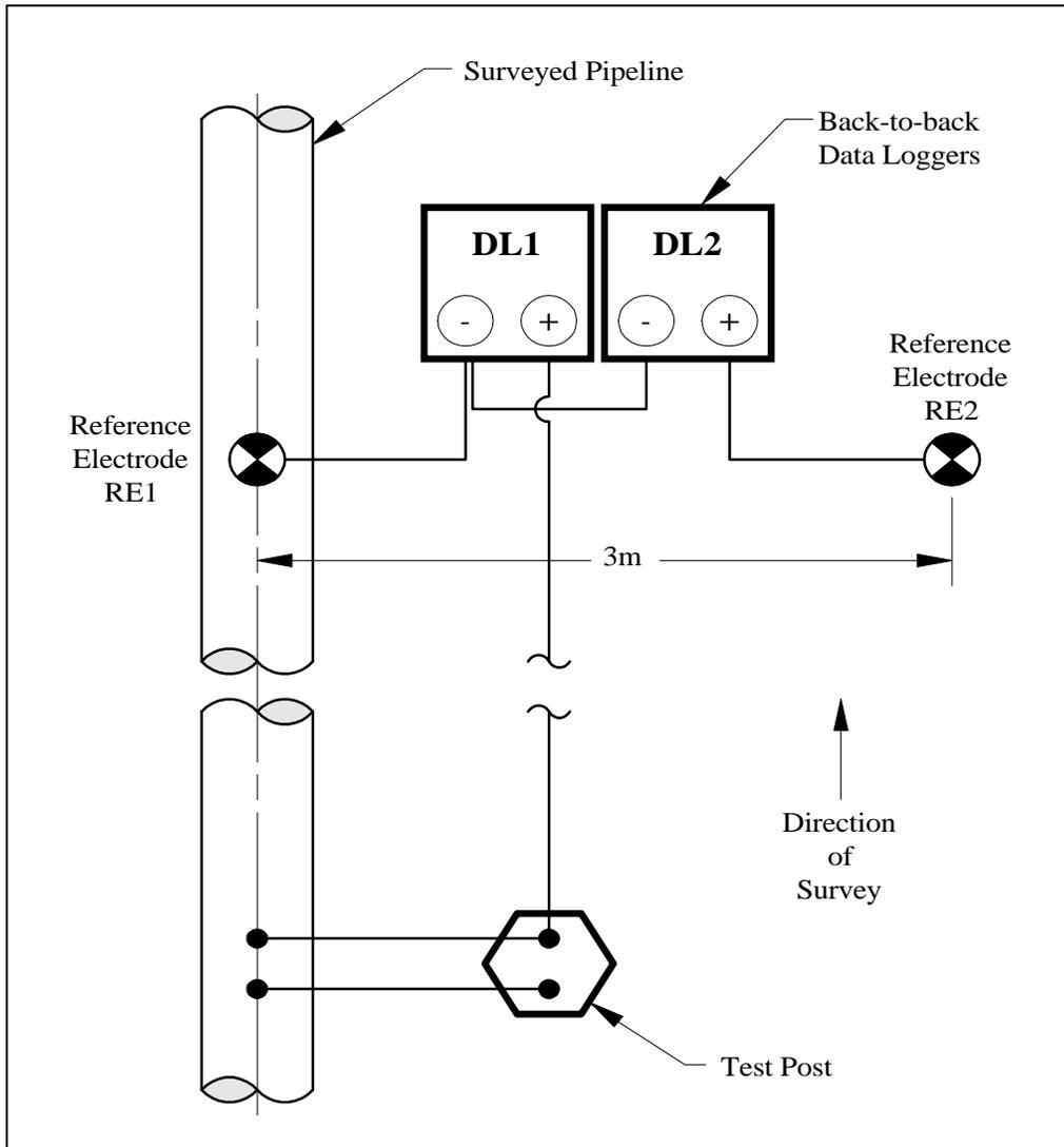
Figure 1. Integrated CIPS/DCVG Arrangement
