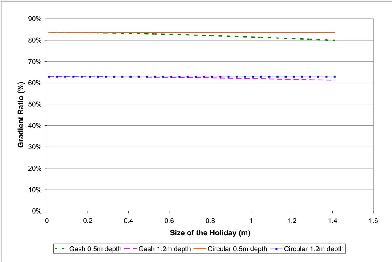
**Figure 5. Variation of the Gradient Ratio  $\left(\frac{\Delta G_{OL-3m}}{\Delta G_{OL-RE}}\right)$  with the Size of the Holiday**
