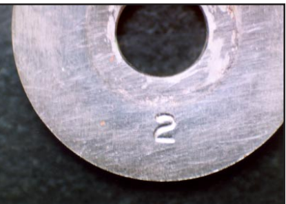
FIGURE 9 • 316L coupon protected by EP system shows no signs of pitting corrosion after exposure in scrubber neutralization tank from January to July, 1997. Small amount of crevice corrosion was visible at the location where isolation washer was situated.
