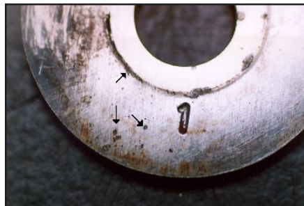
FIGURE 8 • Isolated 316L coupon (control) shows signs of crevice corrosion at the edge where a non-metallic washer was located. The crevice corrosion resulted in a ring above the stamped number “1” as indicated by uppermost arrow. Scattered pitting is shown by the two lower arrows.
