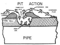
This process continues until the parent metal becomes so flooded with electrons that the positively charged iron atoms can no longer leave the surface because of the attraction of these negative charges.
