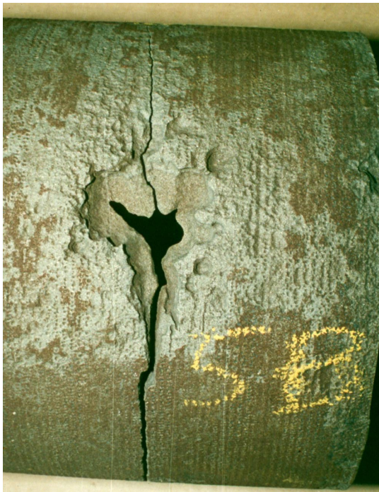
Figure 10 – Cast Iron Break in Figure 4 After Pipe Sample was Sandblasted to Remove the Graphite Corrosion Product
