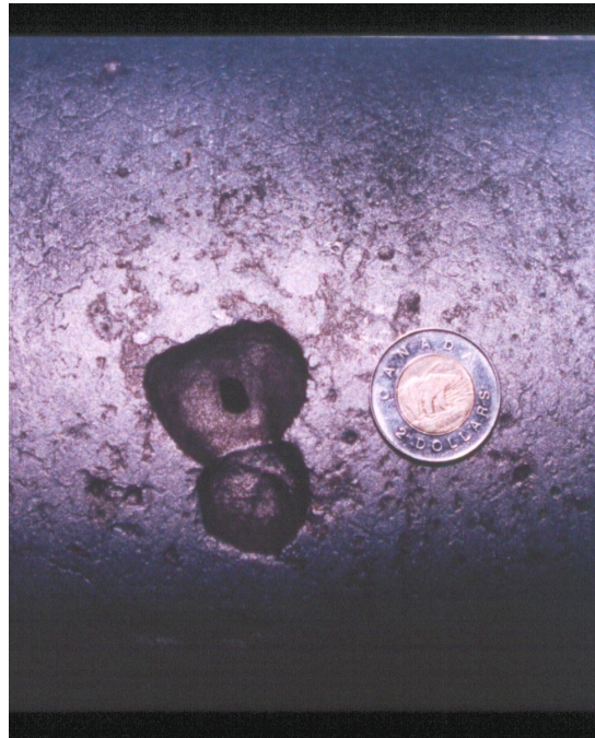
Figure 12 – Typical Corrosion Pit in Ductile Cast Iron
