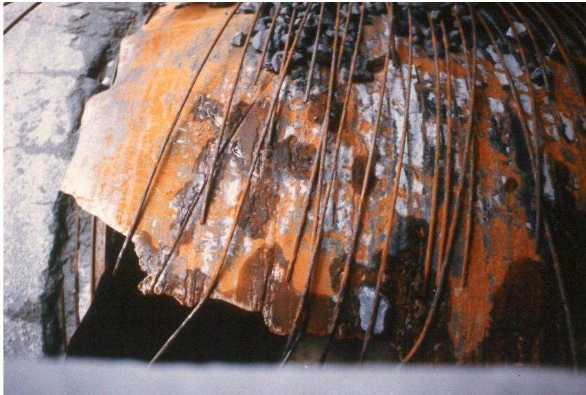
Figure 27 - Typical Corrosion Failure of a Prestressed Concrete Cylinder Pipe
