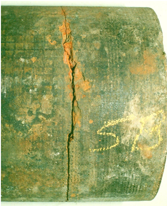
Figure 8 – Typical Beam Break on Grey Cast Iron
