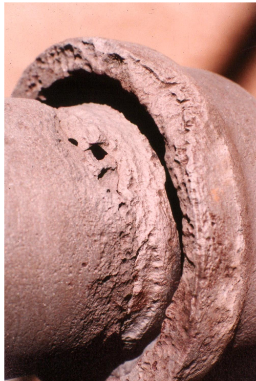
Figure 2 – Stray Current Corrosion at a Bell & Spigot Joint
