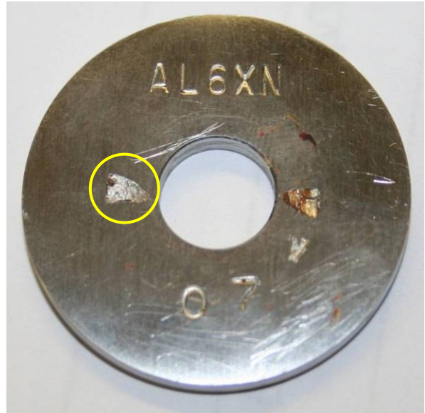
Figure 8b: Unprotected AL-6XN coupon after 15 days exposure. Three visible pits, with a maximum depth of 0.25 mm (250 mpy corrosion rate). Pit circled in yellow is magnified in Figure 8c.
