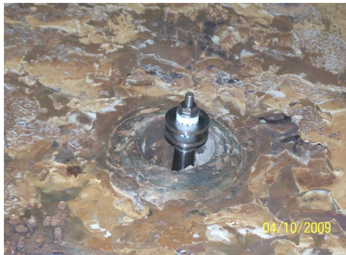
Figure 7: AL-6XN Coupons with Slotted Disk Installed to Gauge System Effectiveness during On-line Operation
