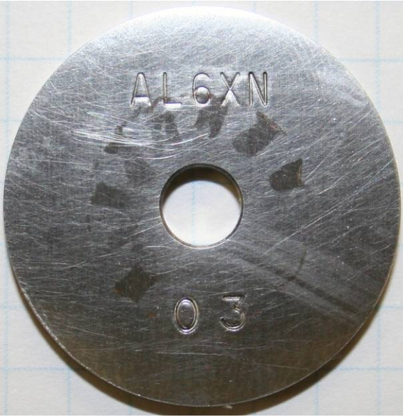
Figure 9a: Protected AL-6XN coupon after cleaning. Slight discoloration where staining and deposits were present; no crevices. 43 day exposure. Coupon dimensions: 1 ¼ inch dia.; 1/8 inch thick
