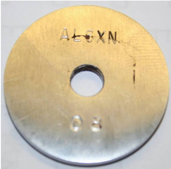
Figure 8a: Protected AL-6XN coupon after 15 days exposure. No signs of corrosion. Brown lines are stains on coupon. Coupon dimensions: 1 ¼ inch dia.; 1/8 inch thick
