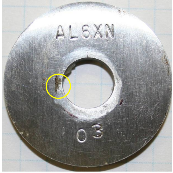
Figure 9b: Unprotected AL-6XN coupon cleaning. Stains largely eliminated, pits still visible. Pit circled in yellow is magnified in Figure 9c.
