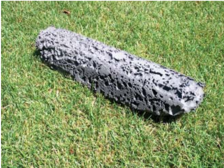
14.5-kg high Mg casting reclaimed from a water main cathodic protection system.
