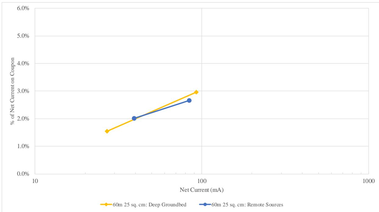
**Figure 4: Effect of remote shallow and local deep groundbeds on a deep coupon**
