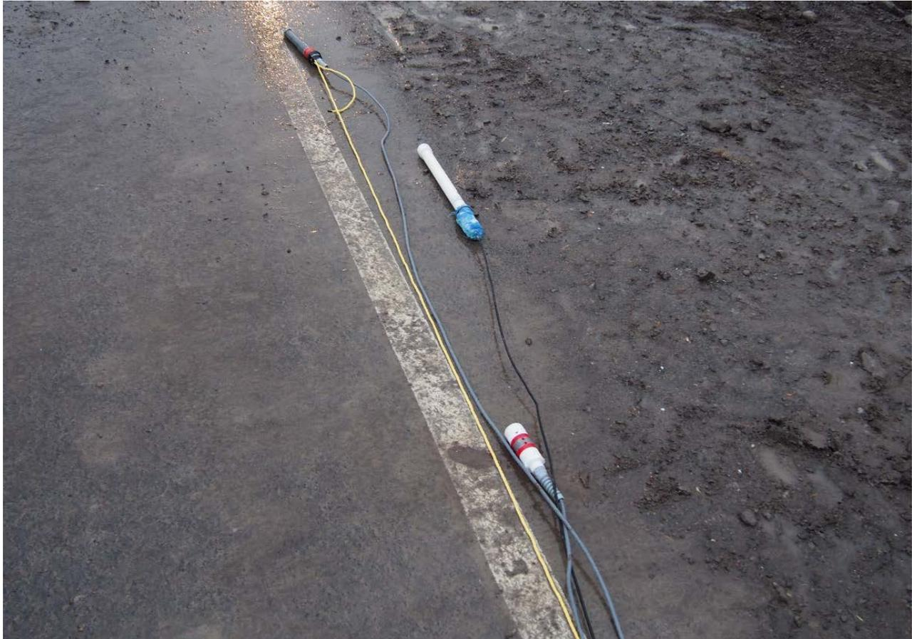
**Figure 1: Coupon assembly consisting of a 10 cm<sup>2</sup> ICR, a stationary CSE and a 25 cm<sup>2</sup> ICR**
