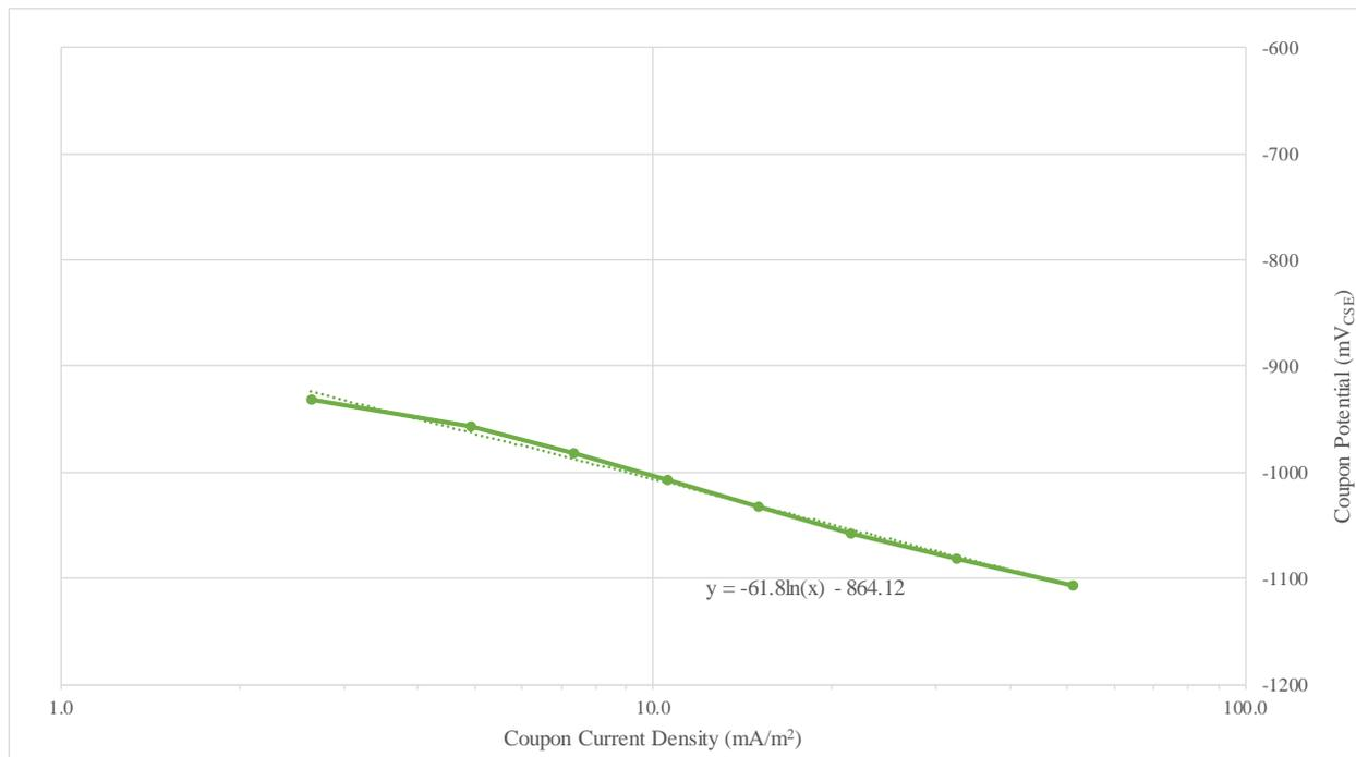
**Figure 6: Polarization curve of coupon in drilling mud**
