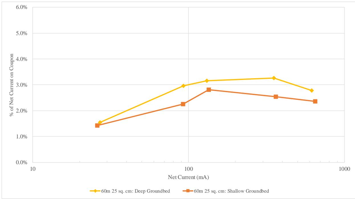
**Figure 3: Effect of local shallow and deep groundbeds on a deep coupon**
