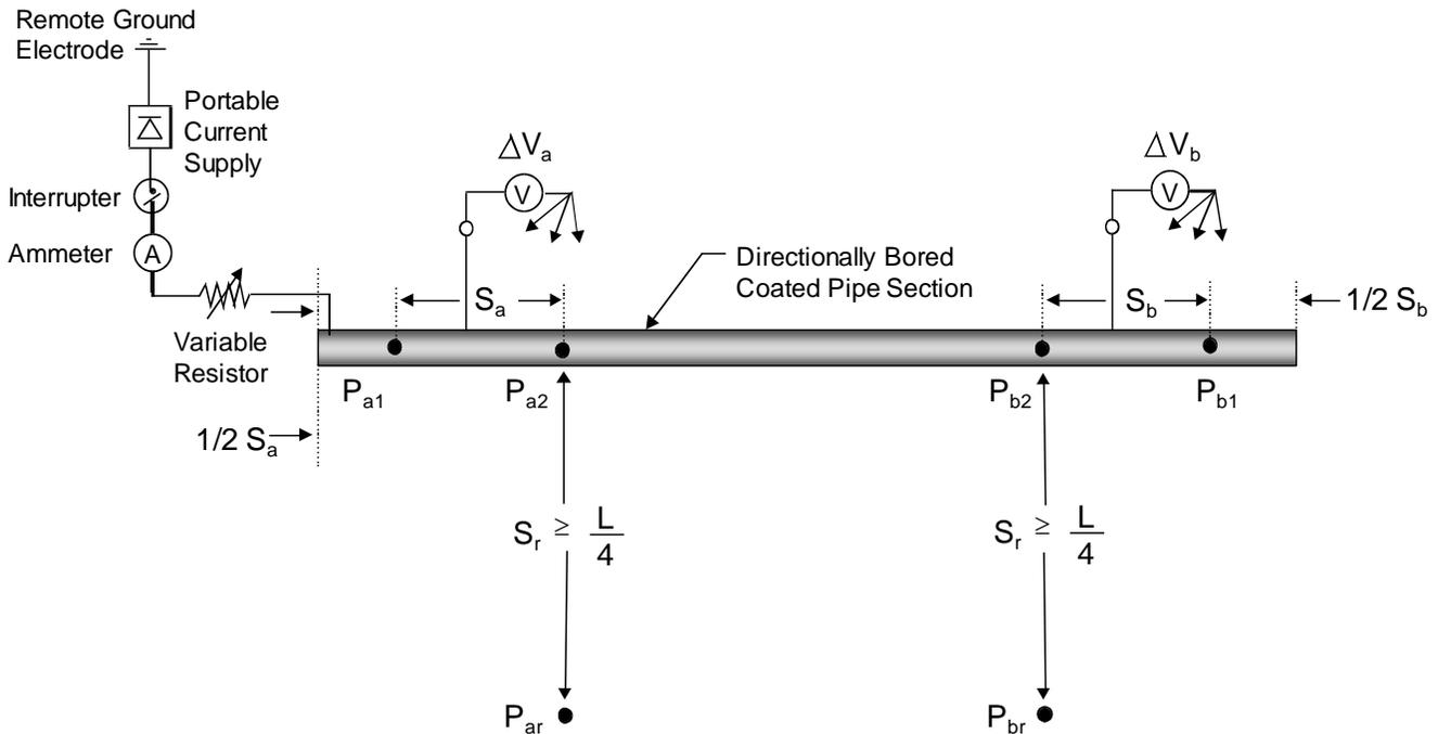
**Figure 2: Arrangement of test equipment and testing schematic**
