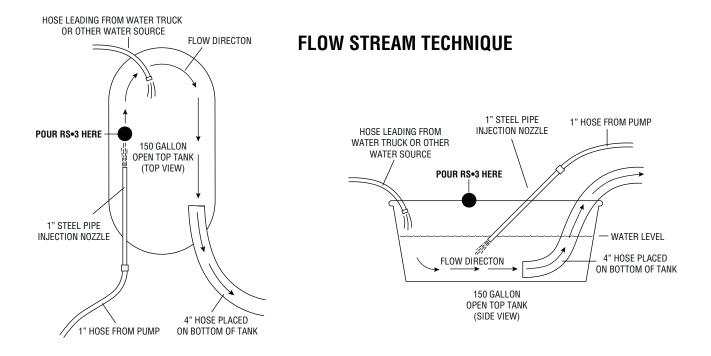
carbon along the tank bottom from the injection nozzle to the suction should be approximately 3 feet (0.9 m) long to allow adequate carbon wetting prior to being swept into the suction. A clean water inlet must also be provided into the top of the wetting tub with an in-line valve for flow control.
