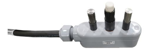
The MEP allows the monitoring of steel embedded within concrete.
