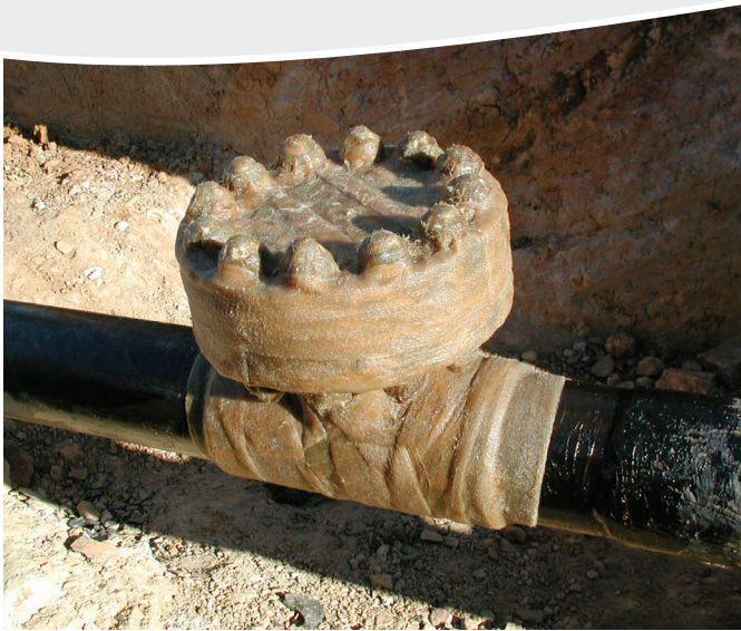
Trenton's Wax-Tape® #1 non-firming anticorrosion wrap protects irregularly shaped underground fittings and is compatible with cathodic protection.
